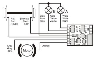
If the bulbs for the directional headlights are floating (isolated against wheel pick up and chassis) and connected according to above figure, they will shine brighter compared to using the rail as a common and the directional headlights will function while operating on conventional DC layouts.
